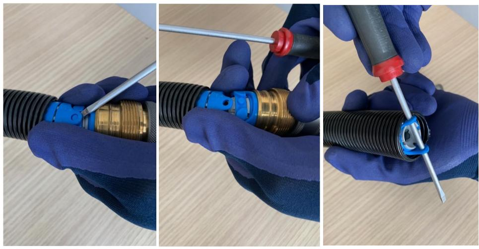
Disconnect the inner body and lock the maxi flex with a tiny screw-driver
