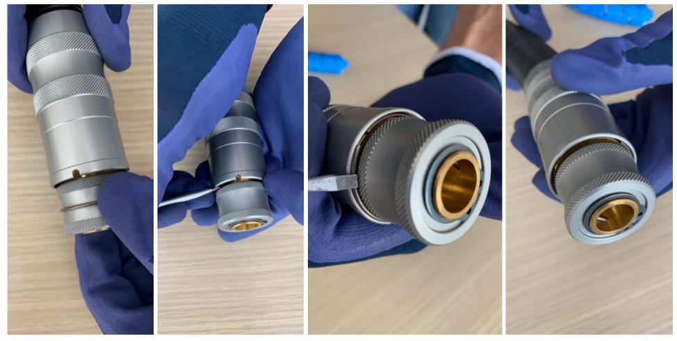
Insert the C shaped locking ring, push it home with a scre-driver, and turn the cap until it locks
