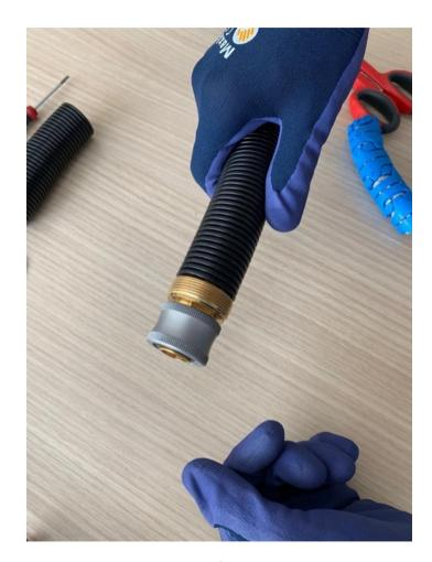
Push the corrugated hose onto the connector rims, as far as it can go
