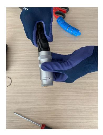
re-wind the outer connector cap
