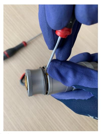
Remove the C shaped locking ring
