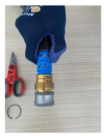
Remove the quick connector cap
