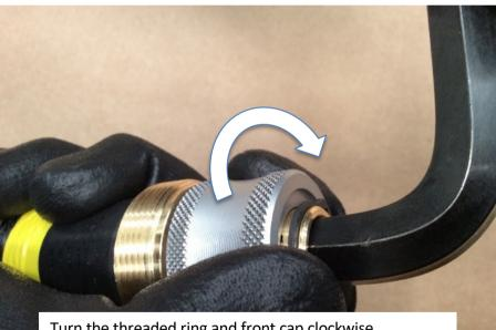
Turn the threaded ring and front cap clockwise. Do not turn the allen key.
